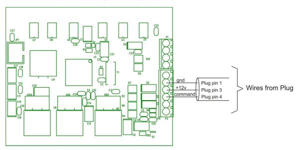
It's suggested to use two separate cables: one with 2 wires twisted and shielded for microphone Another cable with 3 wires twisted and shielded for the display.
